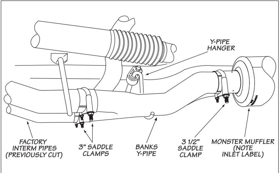
**12.** With the exhaust positioned properly, begin to evenly tighten the clamps starting with the ones closest to the front of the vehicle and working your way back. Torque the exhaust clamps evenly to 35 ft-lbs. Make sure that each slip is fully inserted (+/-1/4").
